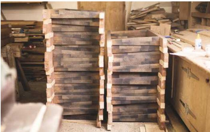
The machined frame segments stack up, fresh from the modified thickener
